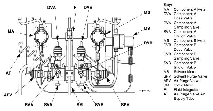
Fig. 67. Wall Mount Fluid Station
